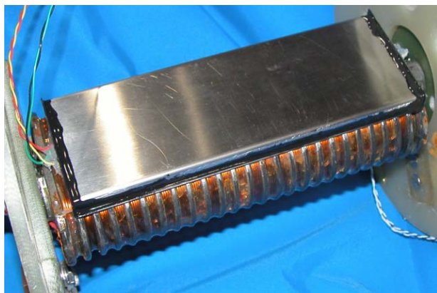
Figure 4: A photo of the vacuum chamber depicted in Fig. 3 (b), attached to the coil/pole face of the SCU before wrapping glass-filament tape around it.
