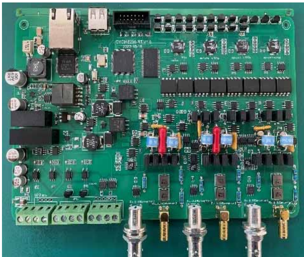
Figure 4: The beam diagnostic electronics for 230 MeV superconducting cyclotron radial probe and scanning wires.
