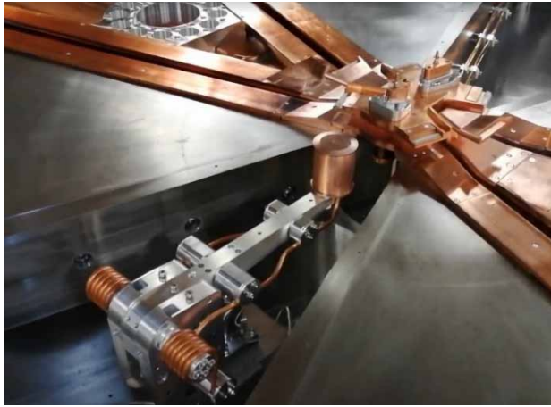
Figure 3. The picture shows the pop-up probe mechanism installed into the valley of the cyclotron.
