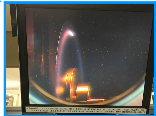
Graphite sheet stripper @ 50 MeV/u
