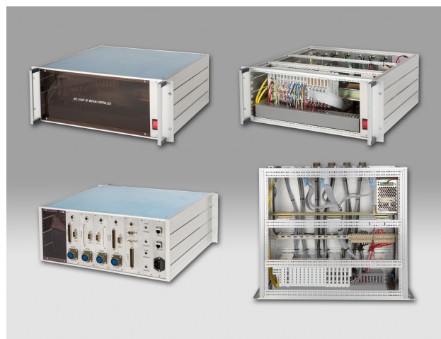
Figure 1: 19-inch rack mountable EtherCAT enclosures designed at iThemba LABS.
