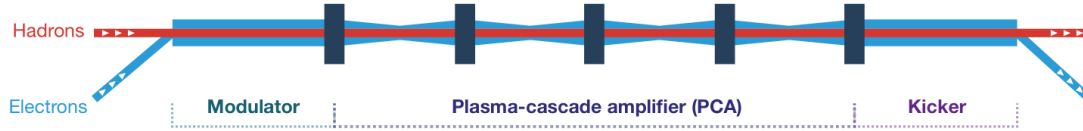
Figure 2: Schematic of a CeC system with the PCA at BNL's RHIC.
