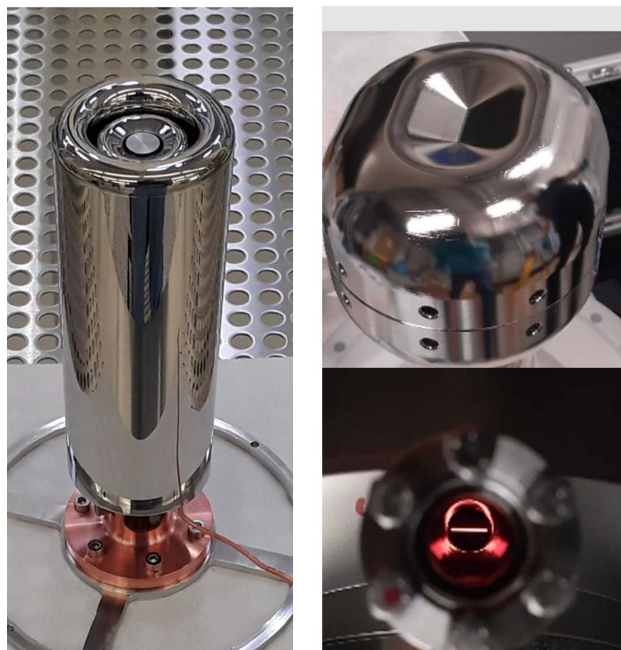
Figure 2: Left: Cathode assembly of the electron cooler test-stand at HIM. Circular cathode with 1 cm diameter. Upper right: Cathode assembly with linear emitter for LFXT. Dimensions 0.3×15 mm. Lower right: emitter in operation.
