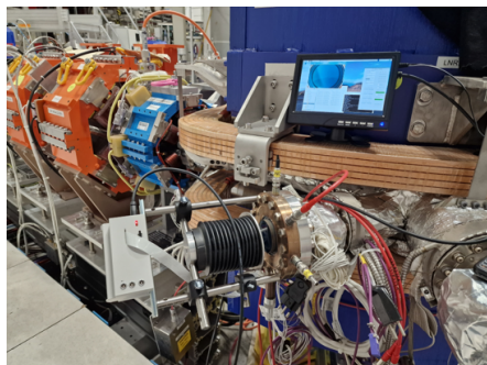
Figure 1: H0 monitor installation
