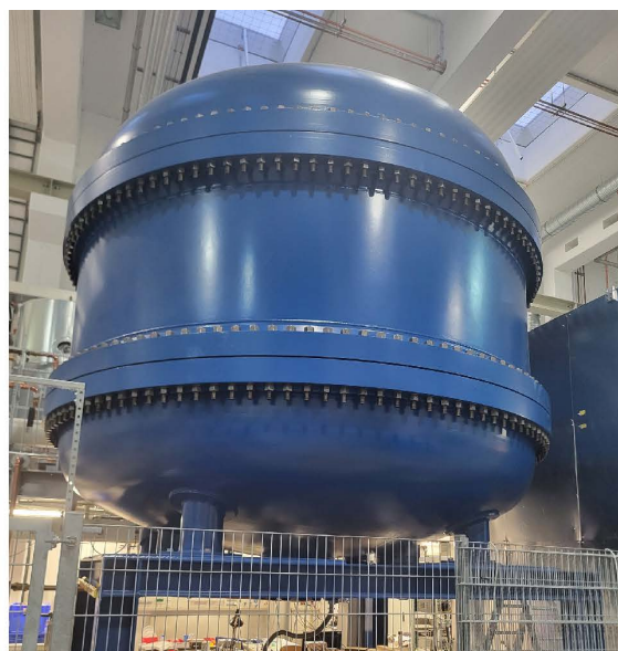
Figure 1: Left: Open tank during assembly of the 600 kV platform which is hanging on a crane. On the upper plane of the platform a solenoid can be identified, the rectangular boxes contain power supplies and communication devices. The right panel shows the tank after tightening all flanges. The inner diameter of the tank is 3.98 m, the outer diameter of the platform is 2.86 m [2].
