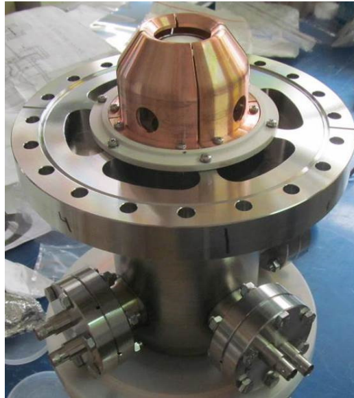
Design of electron gun with 4 sector .
