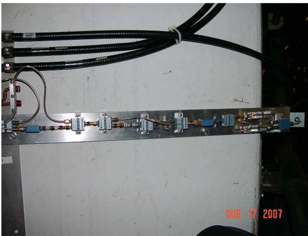
Figure 12: A new equalizer installed in core 4-8 GHz momentum system.
