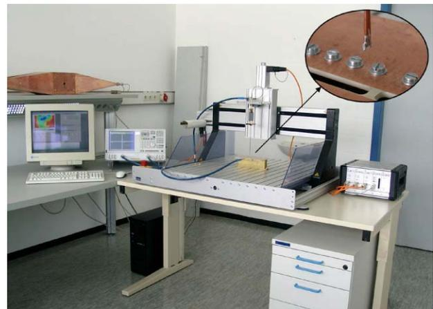
Figure 3: Computer controlled E-field mapper with near field probe (detail).
