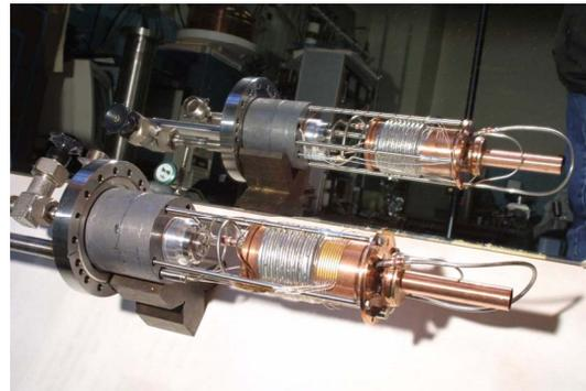
Figure 4: The cryogenic source of slow positrons.
