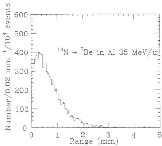
Fig. 8 -- A theoretical simulation of the dose-depth distribution of  $^7\text{Be}$  in Al at 35 MeV/A is shown. Additional nuclear research data will make it possible to compute the dose-depth of  $^7\text{Be}$  in any material.
