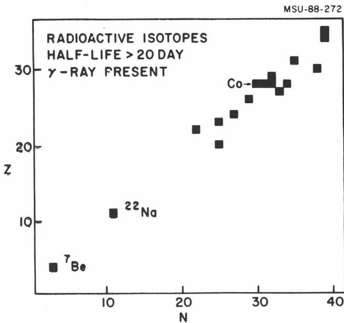
Fig. 1 -- The radioactive isotopes with half-lives >20 days and having a  $\gamma$ -ray in their decay are plotted in a nuclide chart format, i.e. the atomic charge (Z) vs the neutron number (N). Below <40, only  ${}^7\text{Be}$  and  ${}^{22}\text{Na}$  meet the criteria for wear studies.
