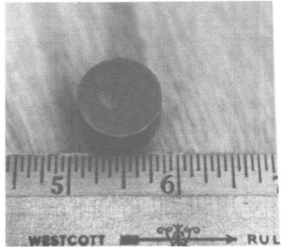
Fig. 9 -- Photograph of the  $\text{Si}_3\text{N}_4$  ceramic disk after implantation of a dose of  $3.7 \times 10^{11}$   $^7\text{Be}$  ions. The disk is 1.91 cm in diameter by 1.27 cm thick. The integrated nitrogen beam current was  $4.2 \times 10^{16}$  particles.
