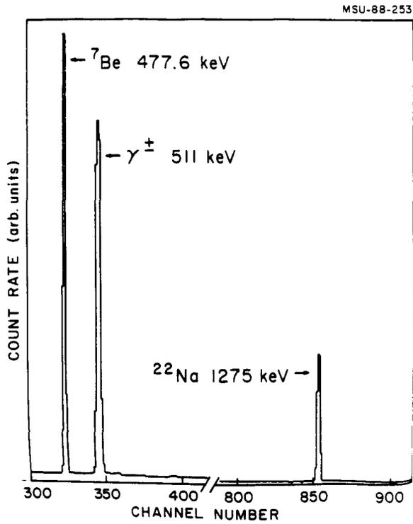
Fig. 4 -- The  $\gamma$ -ray spectrum from an Al foil placed behind the C target bombarded with a 35 MeV/A  ${}^{14}\text{N}$  beam. This spectrum was taken with a 35% efficient Ge detector. Only  $\gamma$ -rays from  ${}^7\text{Be}$  and  ${}^{22}\text{Na}$  are detected.
