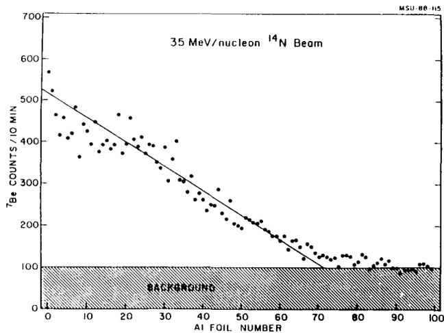
Fig. 5 -- The dose-depth relationship is shown for  ${}^7\text{Be}$  ions implanted in stacked 0.0025-cm thick Al foils for primary  ${}^{14}\text{N}$  beam energies of 35 MeV/A.
