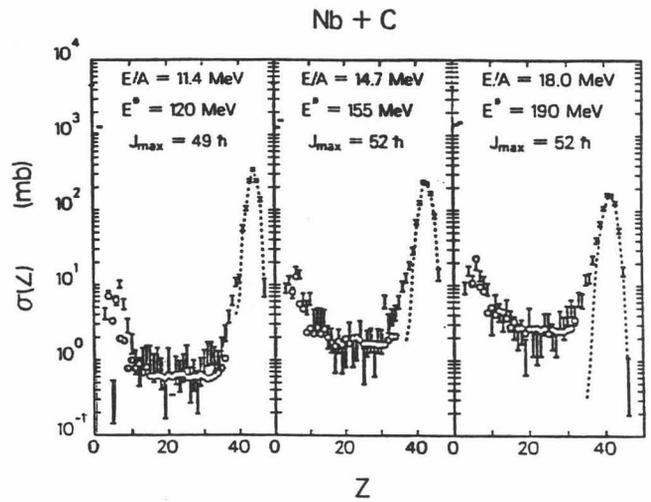
Fig. 2 -- The total cross section for Nb fragmenting on a carbon target is shown for three energies as a function of the fragment atomic number. The bars are experimental data points. The cross-section peaks near the projectile atomic number and for the very light isotopes.
