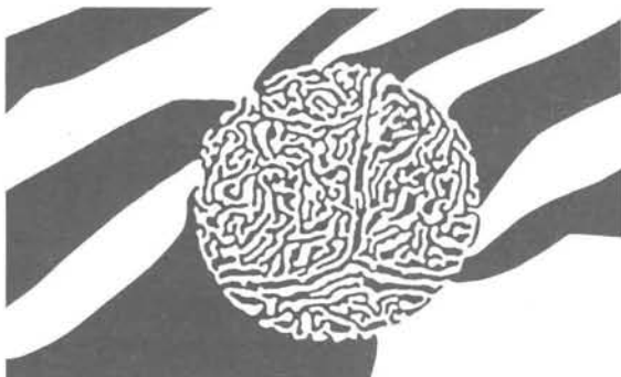
Fig. 18 Effect of etched tracks on the storage density of a magneto-optic film 9) The etched tracks are in the round central region.
