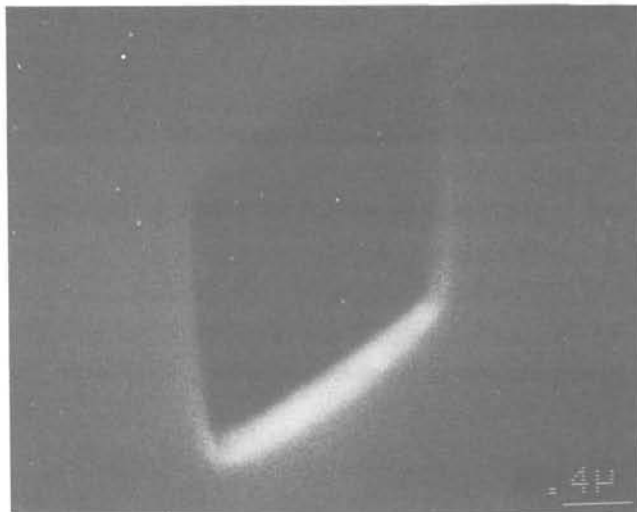
Fig. 10 Cross-section of an etched track in mica.
