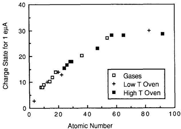
4. Charge states for 1 eµA intensity from the ECR source for gas and solid material feed.
