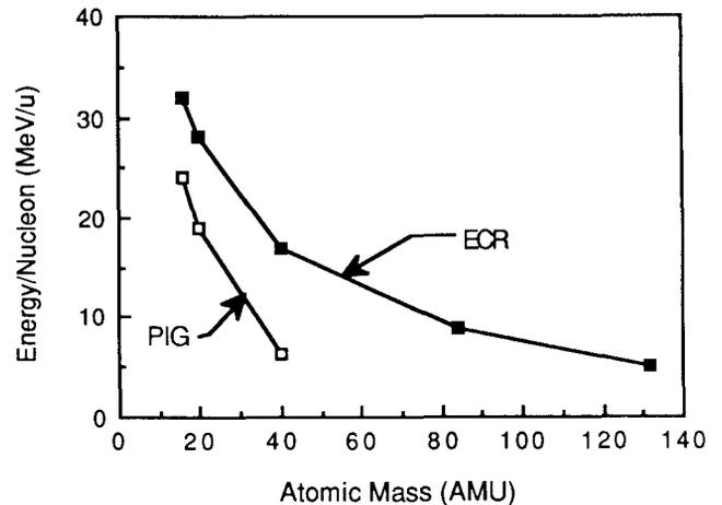
1. Energy vs. mass using PIG and ECR sources, with  $10^{10}$  particles/sec cyclotron external beam.
