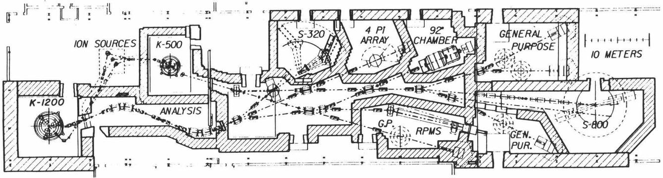
Fig. 2. The highbay floorplan of the complete NSCL Phase II Facility as presently planned; showing the two cyclotrons, the ion source switchyard, the beam transport system to deliver the beam from either cyclotron to any experimental area, and the various experimental devices.
