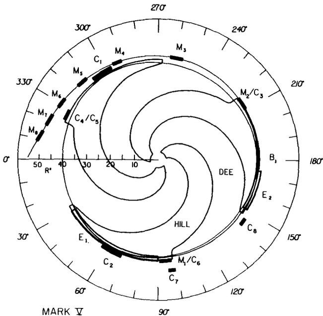
Fig. 1. Section view of the median plane of the K1200 cyclotron. For scale, the outside diameter of the cryostat, the largest circle shown, is 2.9 m. The outside diameter of the steel yoke (not shown) is 4.4 m.
