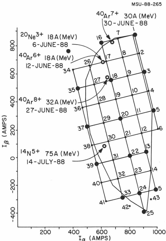
Fig. 3. An operating diagram of the K1200 cyclotron in the space of the two main coil currents,  $I(\alpha)$  and  $I(\beta)$ . The numbered grid points were proposed field maps, with the bold points being the ones mapped to date. The labelled stars are the operating points for the beams extracted during the commissioning period.
