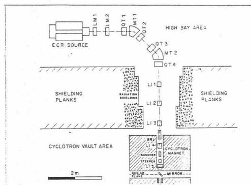
A room temperature ECR source and the injection line are being developed for VEC for obtaining heavy ion beams in 1991.
