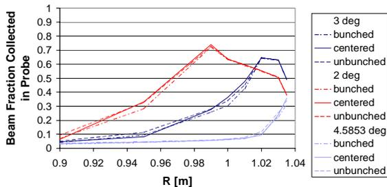
Figure 3: Comparison of calculations with 2.0, 3.0, and 4.5 degree probe heads. The calculations show a greater variation of efficiency at radii lower than the peak, compared with radii greater than the peak.
