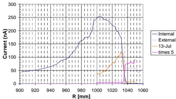
Figure 4: Comparison of a radial probe trace taken with the new 3.0 degree probe head, compared to one taken with the old 4.5 degree probe head.
