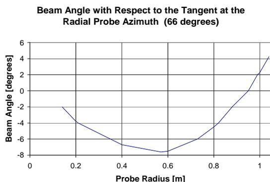
Figure 1: Angle of the C235 proton beam as a function of probe radius, at the azimuth of the probe, expressed relative to the tangent at that radius. Positive angles are scalloping inwards.
