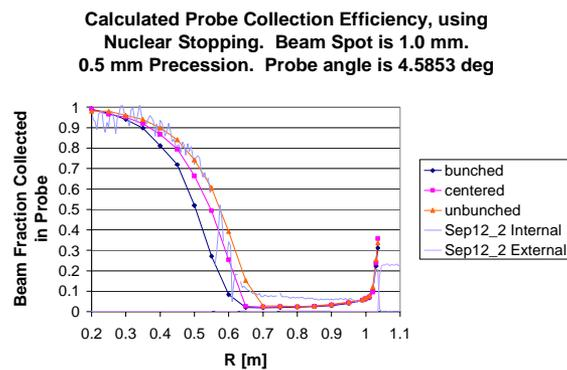
probe traces with the 4.5 degree probe head.
