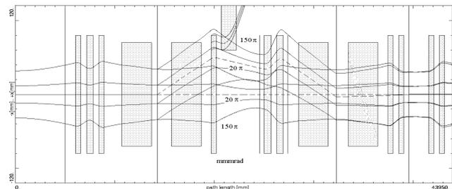
Figure 2: Injection orbit and beam envelope of MMI
