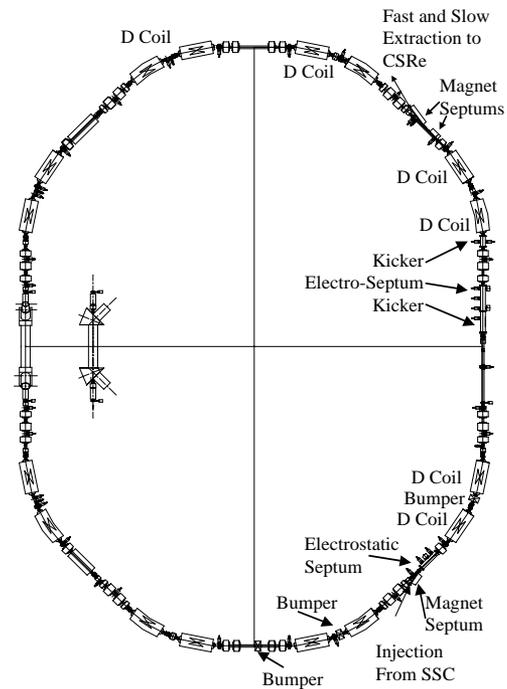
Figure 1: Layout of CSRm injection and extraction
