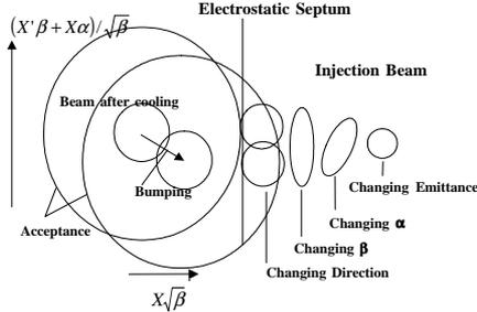
Figure 3: Factors affects gain factor of multiturn injection
