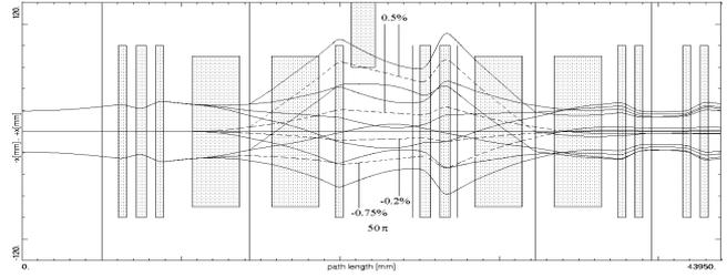
Figure 4: The horizontal beam orbit distribution for RFS
