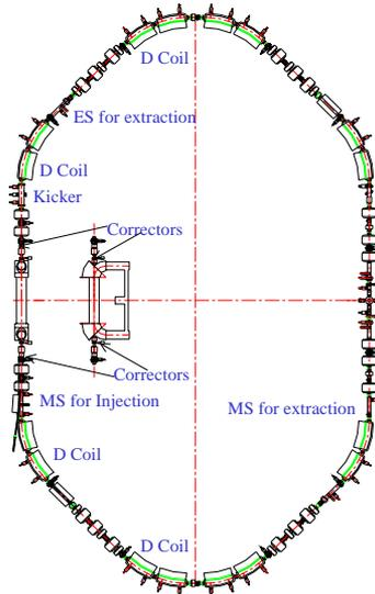
Figure 7: Layout of CSRe injection and extraction
