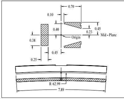
Figure 1: The K1200 injection focusing bar configuration.
