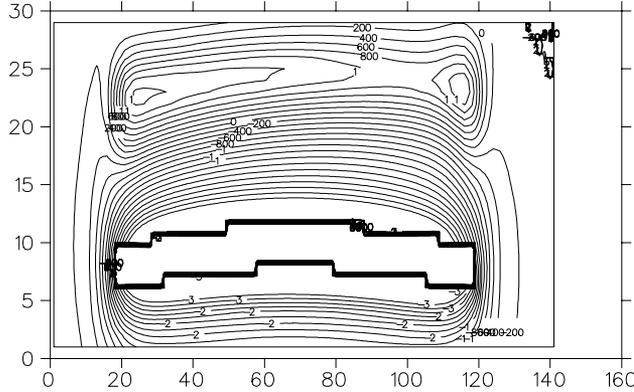
Figure 2: The magnetic field contours of the K1200 injection focusing bar.
