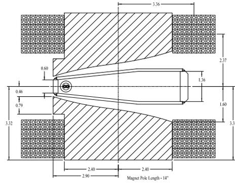
Figure 4: The K1200 injection channel magnet configuration.
