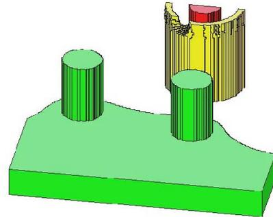
Figure 2: View of the grid used in Relax 3D to determine the electric field near the chimney. Special effort was taken to accurately represent the shape of the source hole.
