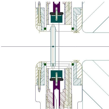
Figure 1: CAD drawing of PIG ion source.
