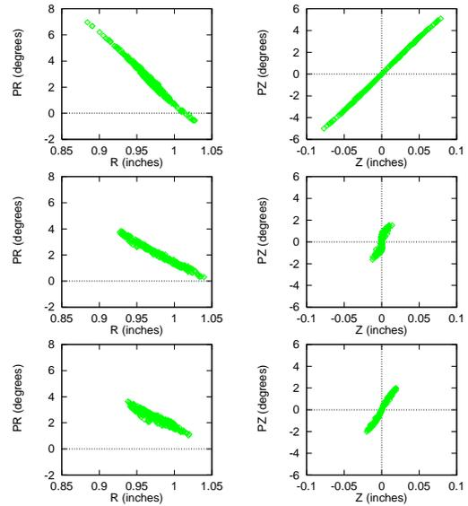
Figure 5:  $r - p_r$  and  $z - p_z$  phase space diagrams for the three different plasma boundaries shown in figure 3. A and B are the  $r - p_r$  and  $z - p_z$  for a concave plasma boundary. C and D are for a slightly convex plasma boundary, and E and F are for a very convex plasma boundary.
