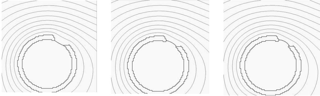
Figure 3: In each image, the dark line represents zero potential. The dark line that goes across the source exit hole is taken to be the “plasma boundary,” the starting point for each ion. The three different plasma boundaries were produced using different values for the image electrode.
