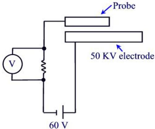
Figure 8: Electrical circuit used to measure the beam current that hits each of the probes. The entire circuit floats at 50 KV.
