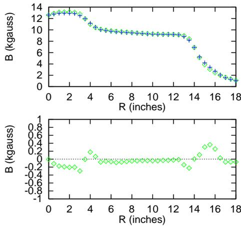
Figure 4: Graph one shows the azimuthally averaged field (Kgauss) as measured (diamonds) and calculated with TOSCA (pluses). Graph two shows the difference between TOSCA and measured fields.
