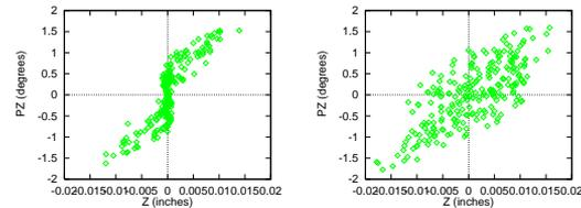
Figure 6:  $z - p_z$  phase space plots for two different starting energies for the ions. The larger the starting energy, the larger the phase space area.
