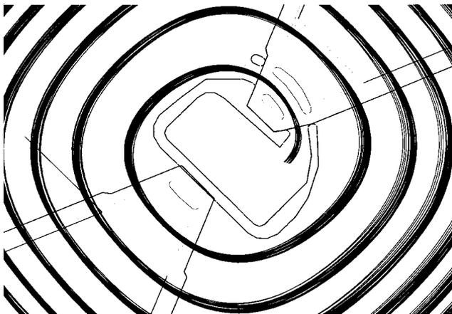
Figure 4. TENSOR Central region. Presented trajectories of 20 RF deg phase band and normalized emittance  $0.5 * \text{PI mm} * \text{mrad}$ .
