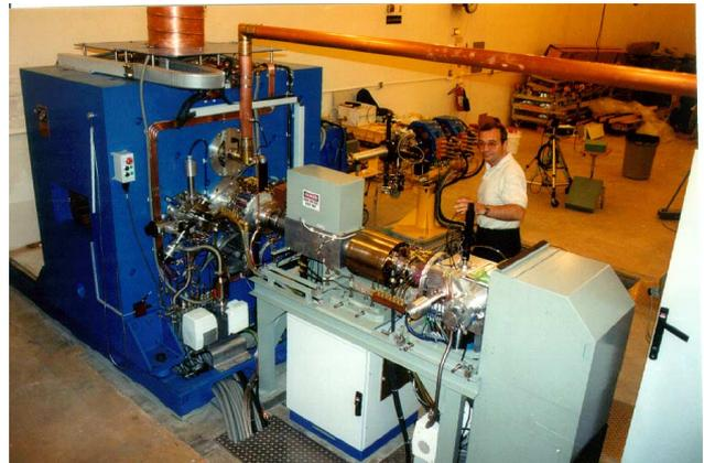
Figure 1. TR9D Assembly. Injection line, Magnet, Beam line.
