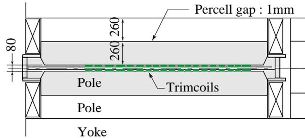
Figure 2: Cross-sectional view of the pole and the beam chamber of the sector magnet. Grey area shows the parts treated as one unit.
