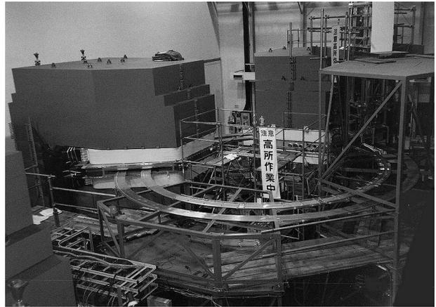
Figure 3: Photograph of the two sector magnets and the magnetic field mapping device at Sumitomo Heavy Industries, Ltd. in Ehime prefecture.
