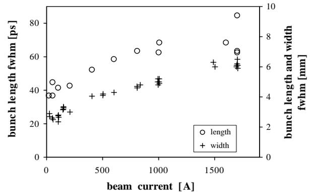
Figure 2: Phase width and radial width of beam bunches, measured at extraction from PSI Injector 2 for different beam intensities [8].
