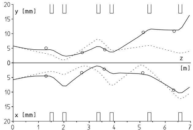
Figure 1: Transport envelope fit in 870 keV beam line. Solid: best fit with space charge effects; 14% neutralization yielded the best result among the runs with different values of this parameter. Dashed: envelopes with zero space charge effects, but same initial condition.
