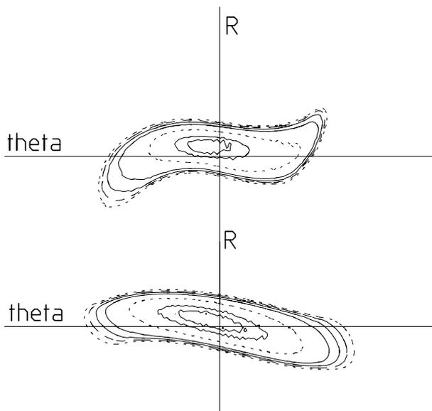
Figure 3: Charge density distributions of a beam bunch on the first turn of Injector 2. Above: Simulated with radial collimation of a wide phase beam. Below: Produced with standard initial conditions of the program PICN.
