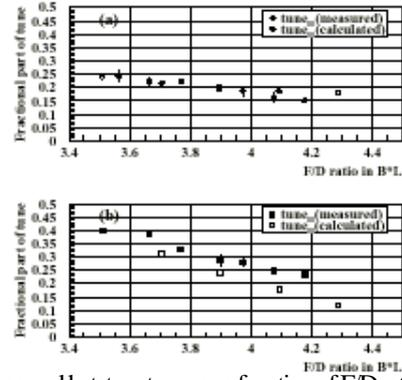
Fig 4. Measured betatron tunes as a function of  $F/D$  ratio.
