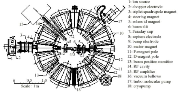
Fig 2. Photograph and schematic layout of the POP FFAG machine.
