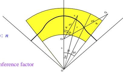
Fig 1. Linearized orbit configuration of a triplet radial sector (DFD) type of FFAG.
