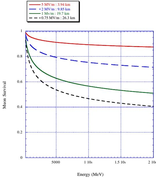
Figure 8. Muon survival during acceleration from 300MeV/c to 20GeV/c for various accelerating gradients and fractional distances along the machine.
