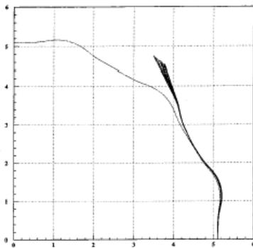
Fig 9. Typical extraction orbit of 150MeV FFAG operation
