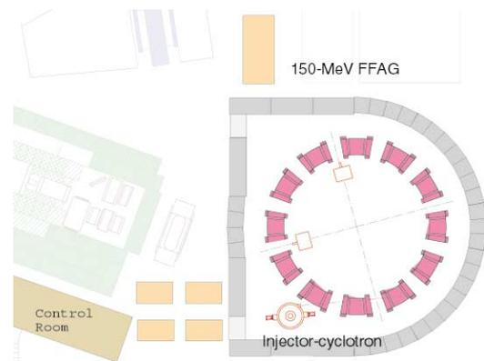
Figure 7. Schematic view of the 150MeV FFAG
