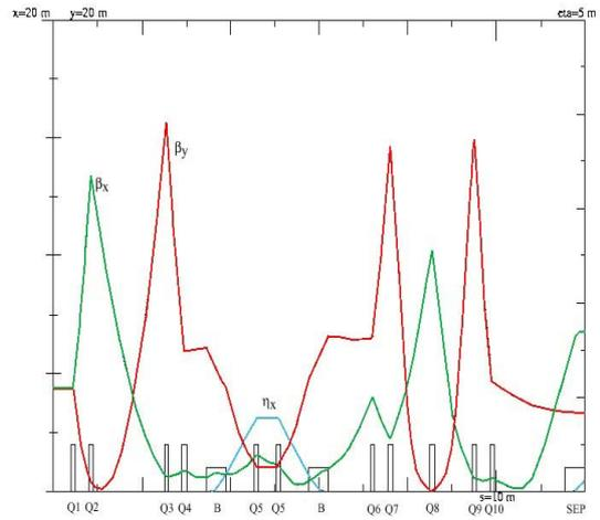
Figure 2. The beam optics of LBT
