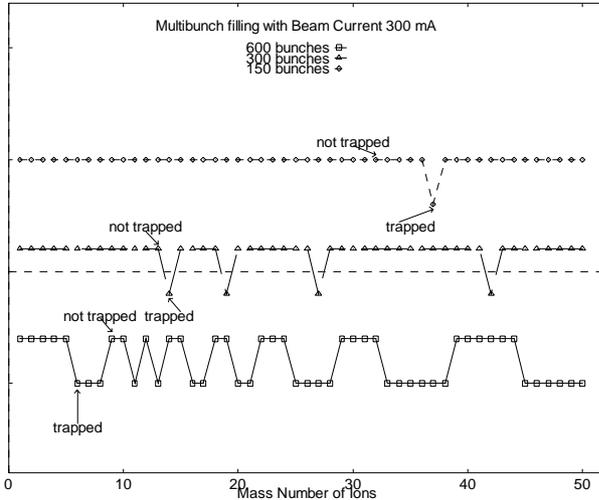
Figure 2: Ion stability for continuous multi-bunch filling with total beam current 300mA (a) 600 bunches, (b) 450 bunches, (c) 300 bunches, and (d) 150 bunches.
