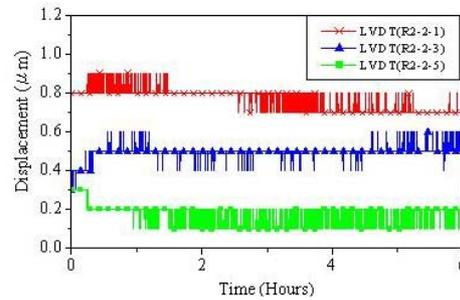
Figure 6: Minimize the girder height change by reducing the chamber expansion effect. (2001/8/21)
