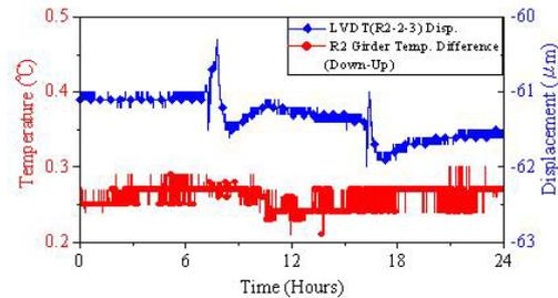
Figure 3: The temperature difference of the girder and LVDT data after insulation. (2001/8/28)
