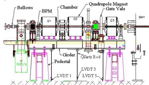
Figure 1: The girder assembly and layout of LVDT
