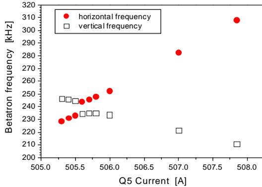
Figure 4: Closest tune approach for coupling measurement. (Sep. 4, 2001)
