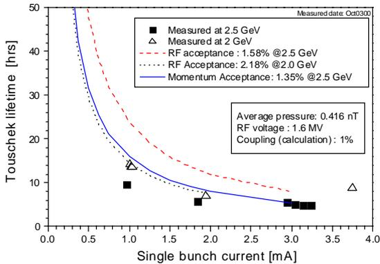
Figure 5: The measured Touschek lifetime as a function of single bunch current (Oct. 04, 2000).
