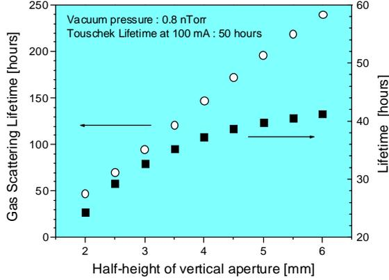
Figure 2: The calculated gas scattering lifetime and lifetime as a function of half-height of vertical aperture.
