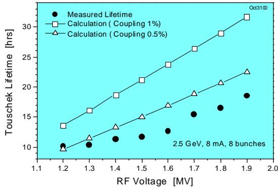
Figure 3: The measured and calculated Touschek lifetime as a function of RF voltage.
