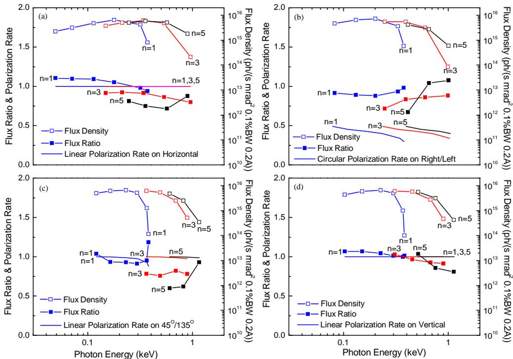
Figure: 2 Photon flux density, flux ratio, and polarization rate are calculated at distinct polarization modes, (a) horizontal polarization (phase  $\theta=0$ ), (b) elliptical polarization (phase  $\theta=1.131$ ), (c) linear polarization,  $45^\circ/135^\circ$  (phase  $\theta=1.822$ ), (d) vertical polarization (phase  $\theta=3.141$ ).
