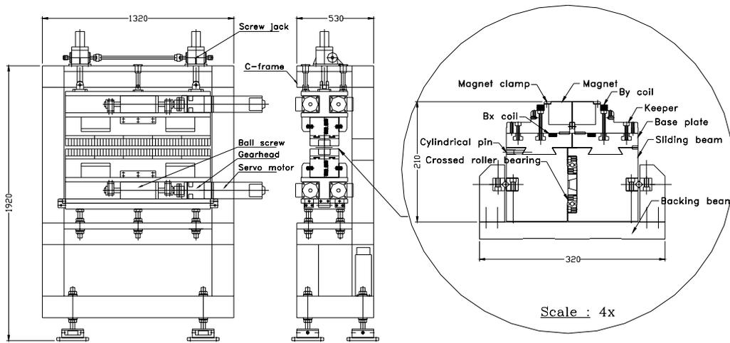
Figure: 1 The overall design of the prototype one-m-long elliptical polarization undulator.
