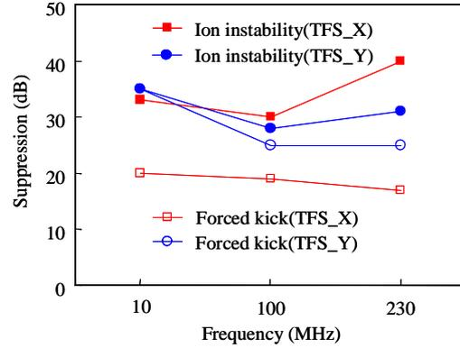
Figure 2: Suppression of betatron sidebands plotted for feedback on
