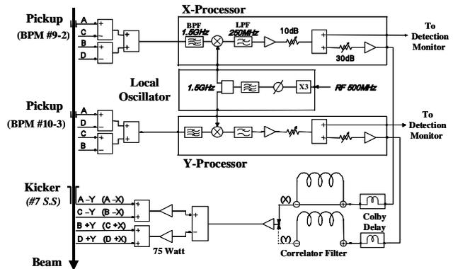
Figure 1: A layout of the transverse feedback system
