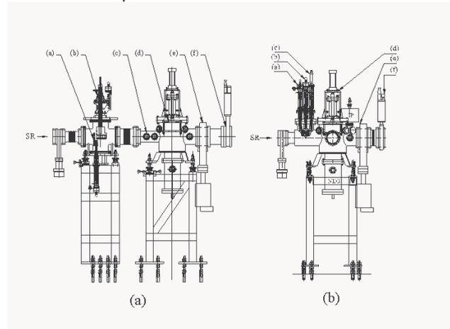
Figure 1: Layout of front ends for (a) Insertion Device (ID), and (b) Bending Magnet (BM) sources for the TLS. The main components for the front ends contain (a) aperture, (b) PBPM, (c) absorber, (d) safety shutter, (e) metal gate valve, and (f) fast closing shutter.
