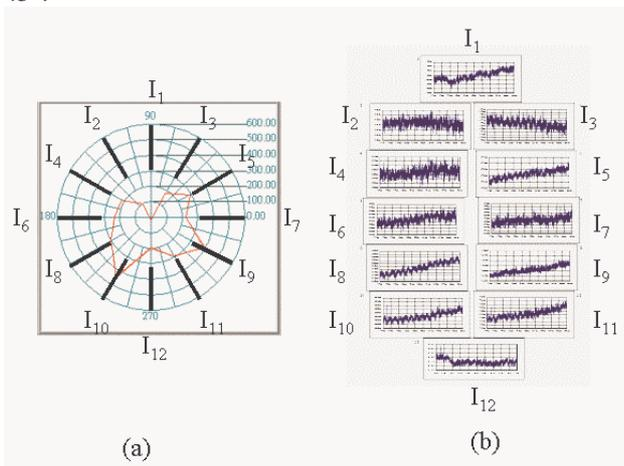
Figure 7: Curves of the group signal of 12 sets of blade current normalized to the e-beam current, (a) the radar plot, and (b) the individual current.
