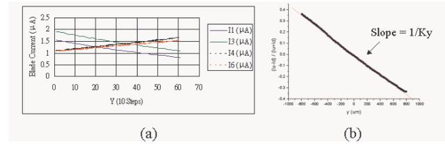
Figure 4: Calibration of  $K_y$  factors for 4-blade PBPM, (a) the curves for the four blades during the vertically moving of PBPM, (b) the curve of the differential blade current vs. the PBPM movement.
