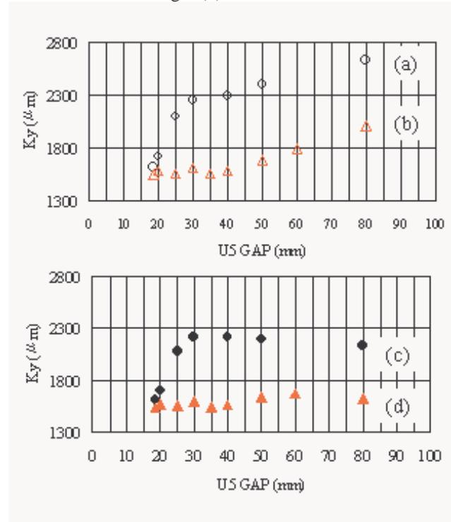
Figure 5: Curves of  $K_y$  factors for 4-blade PBPM for U5 undulator at various open gaps. Where curves (a) and (b) are  $K_y$  obtained without subtracting the BM light when PBPM is located  $\sim 4$  mm offset and at the beam center, respectively. Curves (c) and (d) are  $K_y$  obtained with subtracting the BM light when PBPM is located  $\sim 4$  mm offset and at the beam center, respectively.
