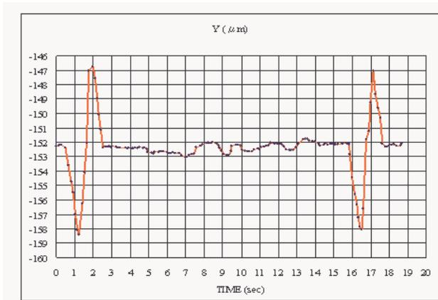
Figure 6: Curves of vertical position, Y, measured at a BM-front end when the electron beam subjected an anomalous periodically driving force.
