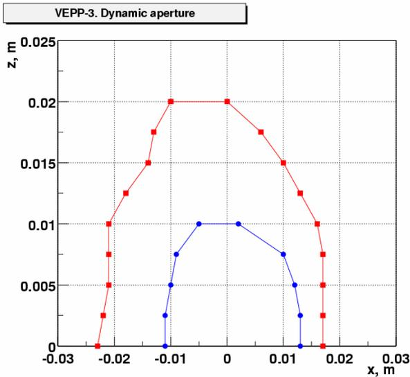
Fig. 4. Dynamic aperture for non-perturbed (external points) and perturbed (internal points) lattices of storage ring VEPP-3.
