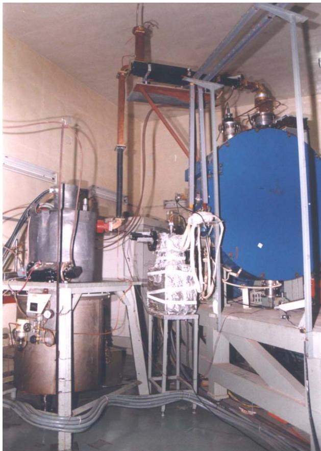
Figure 3: Photograph of assembly of the 5MW klystron and waveguide line with the Injector Microtron. On the back side is shown the klystron modulator.
