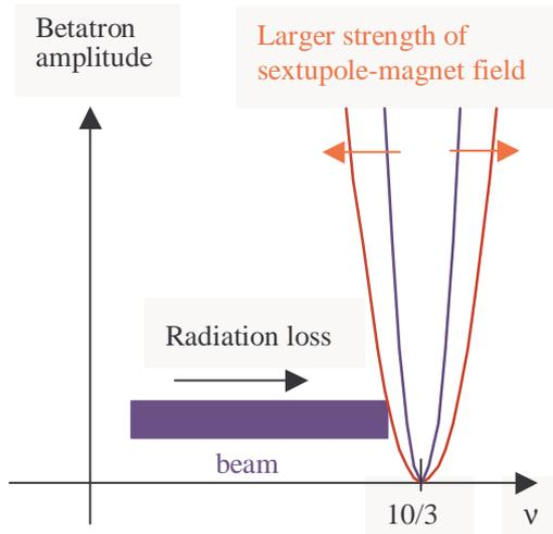
Figure 2: Schematic diagram of beam extraction.
