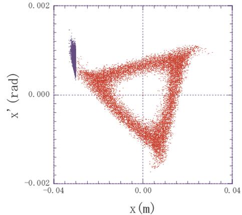
Figure 3: Horizontal phase space distribution at a wire septum. The extracted beam ( $x < -0.03\text{m}$ ) is also shown.
