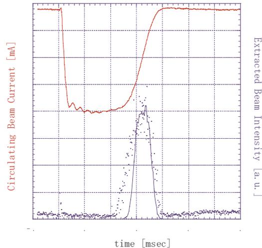
Figure 4: Time distribution of extracted beam. Solid line: tracking simulation, Plot: measured by spill monitor, Upper line: ring current measured by DCCT.
