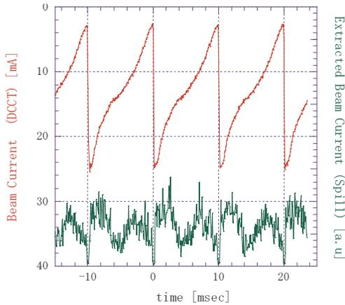
Figure 5: Time distribution of extracted beam for 100 pps operation. A ring current is also shown (upper line).
