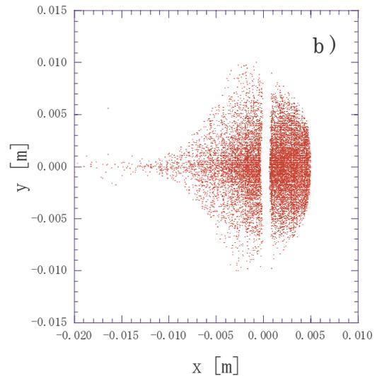
Figure 6: Profile of extracted beam. a): measured, b):tracking simulation
