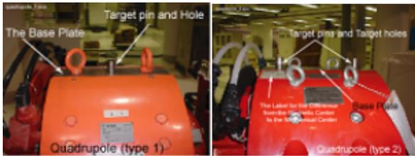
Fig.16 Two types of the quadrupoles
