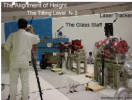
Fig.13 The alignment for the dipole
