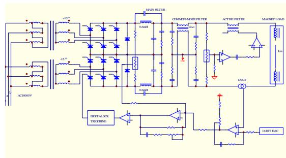
Fig. 1 The dipole power supply diagram
