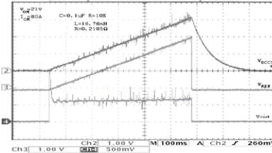
Fig. 7 The output current & error waveform of Q power Supply Prototype ( I<sub>p</sub>=80A, L=17mH, R=0.21 Ω )
