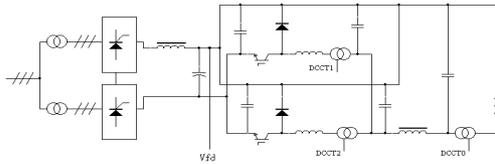
Fig. 2 The Q. magnet main winding power supply
