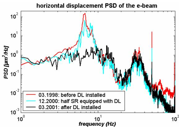
Figure 3: Horizontal displacement PSD of the electron beam before, during and after the installation of the damping links in
