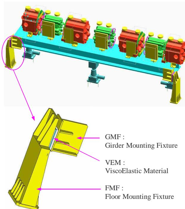
Figure 1: Damping link and installation on a G20 magnet girder assembly in the ESRF storage ring
