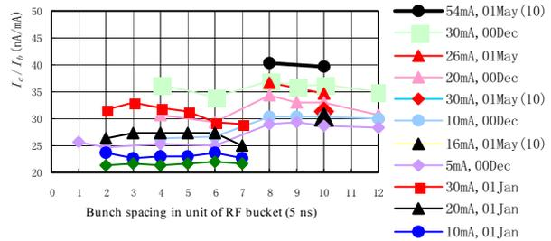
Figure 6: Normalized electron current as a function of bunch spacing and current. The legend gives beam current.
