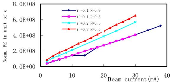
Figure 9: PE creation for different yield and reflectivity. The energy distribution of the SE is  $0 \pm 5eV$ , and the  $\delta_{\max}$  of the SE is 3 in simulation. Simulation results are shown in Fig. 9 and 10.
