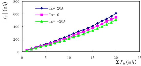
Figure 7:  $I_c$  vs.  $I_b$  with different solenoid fields.
