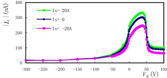
Figure 8:  $I_c$  vs.  $V_b$  with different solenoid fields.
