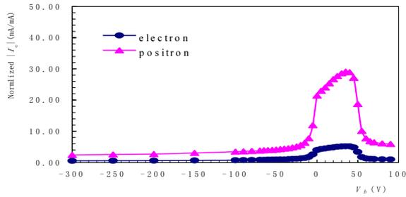
Figure 4: Detector current when bias voltage scans.
