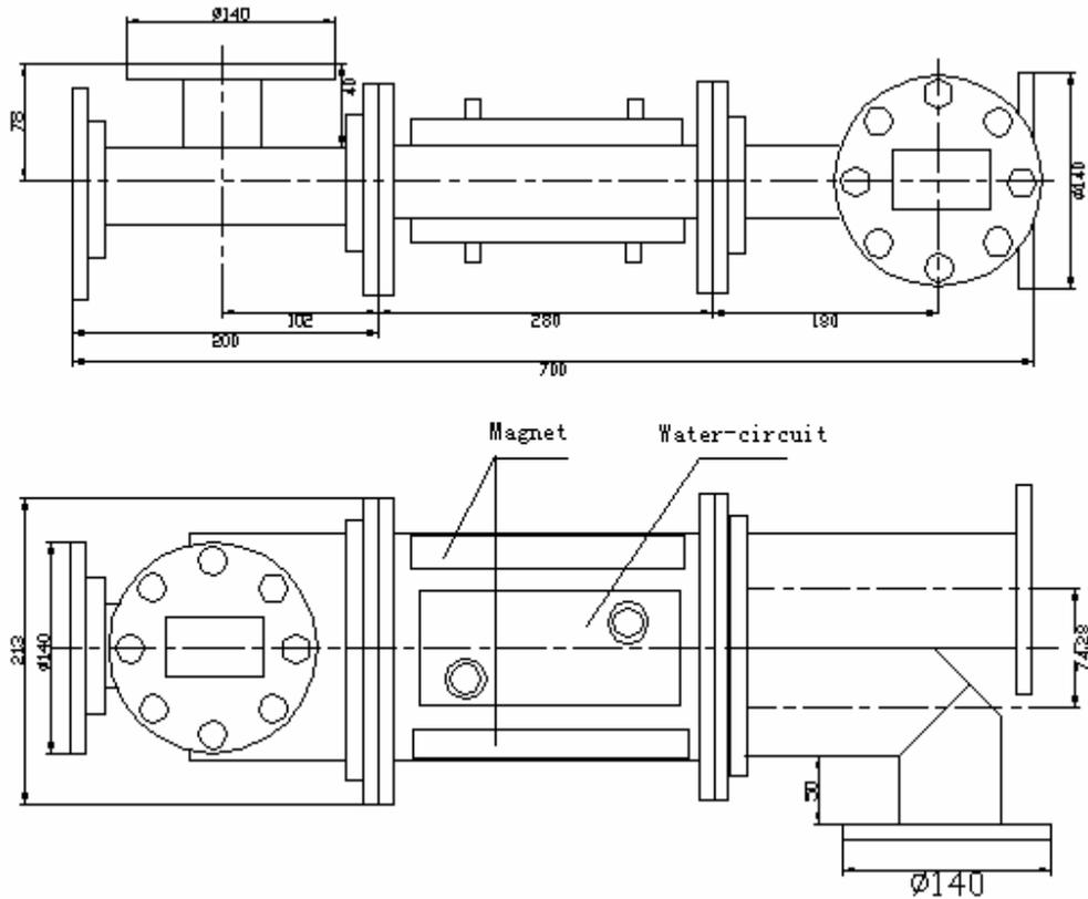
Fig.1 Differential phase-shift circulator
