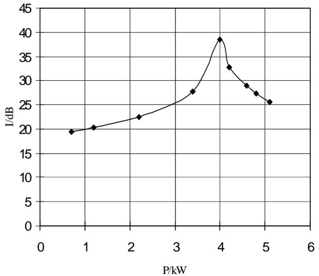
Fig.2 Isolation versus average power at F=2856MHz
