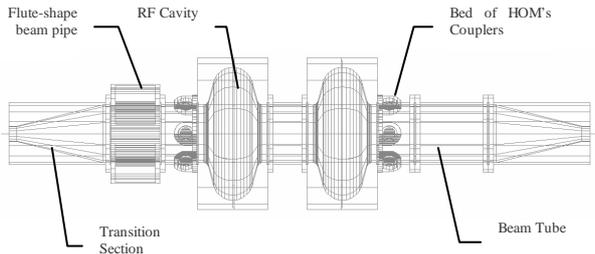
Fig. 1: Layout of A two-cell prototype cavity
