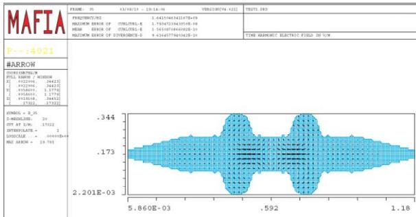
Fig 8: One of the Calculated Double-cell Cavity Modes
