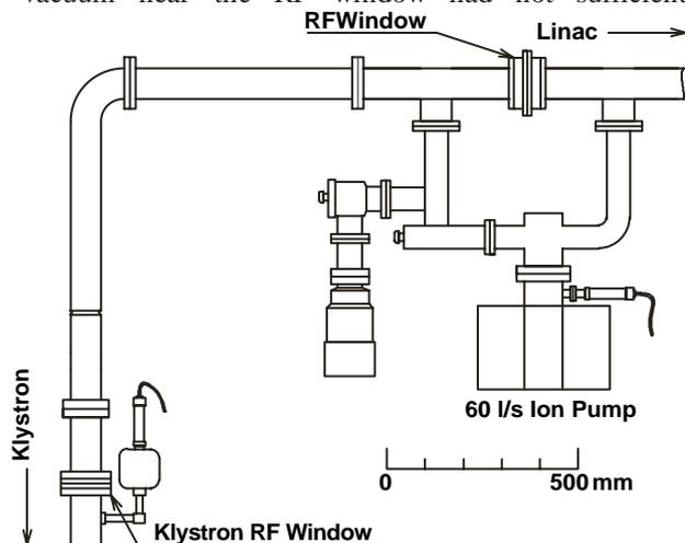
Figure 2. Layout of the waveguide and the vacuum pumping system with a low vacuum conductance.
