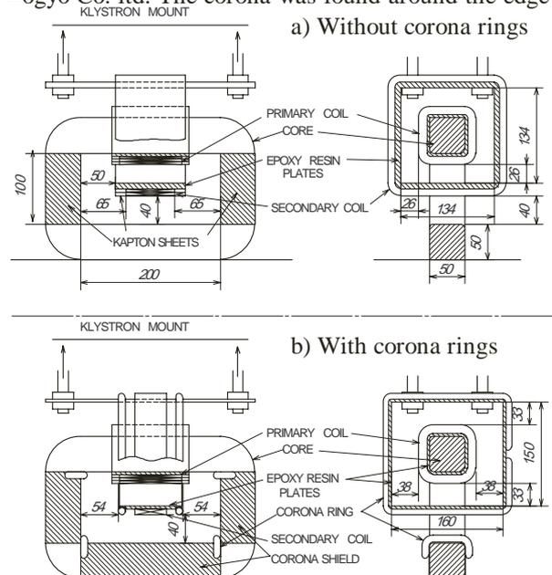
Figure 1. Layout of the heater isolation transformer.
