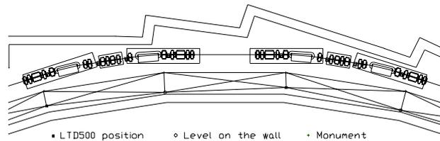
Fig.3: Tunnel network
