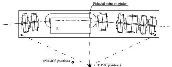
Fig.5 Prealignment for quadruples, sextuple and Bending magnets
