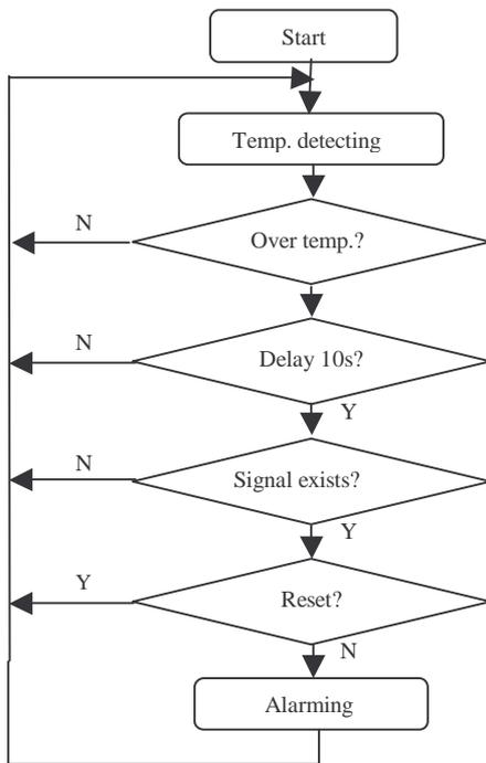
Figure 2: Flow Chart Diagram
