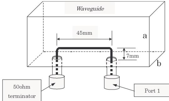
Figure 3: Sketch of the pick-up structure.
