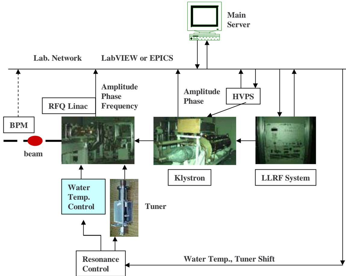
Figure 3. RF feedback loop.
