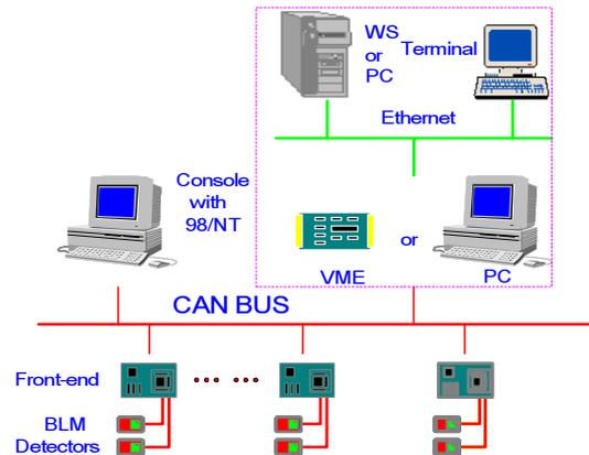
Figure 3: Structure of the BLM System
