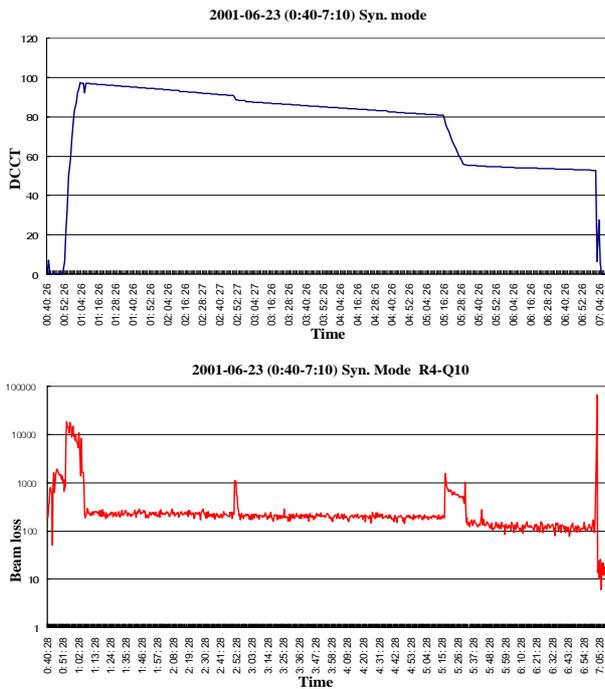
Figure 4: Beam losses on BEPC
