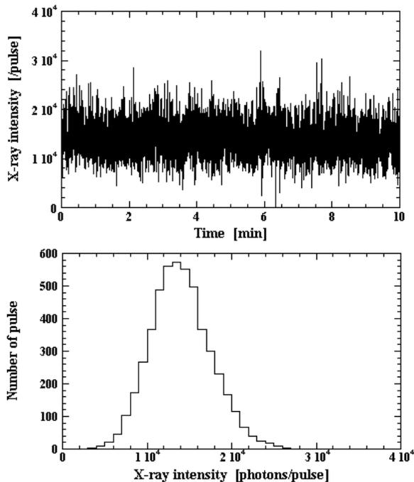
Fig. 4 The pulse-to-pulse fluctuation of the X-ray intensity.
