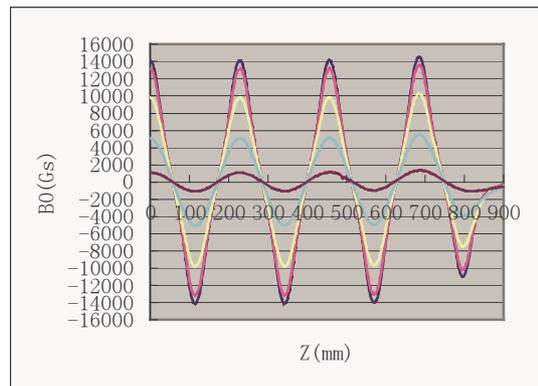
Figure 4: The magnetic field distributions at the midplane of 1W1
