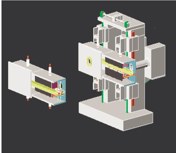
Figure 7: The 3D sketch map of in-vacuum wiggler(4W2)
