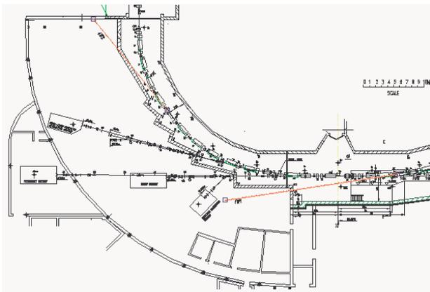
Figure 3: layout of new wigglers in BEPC
