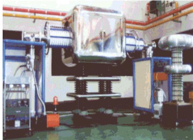
Figure 1: Photograph of the millimeter-wave FEL
