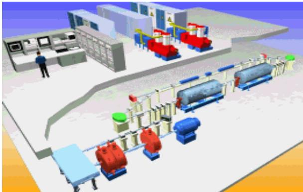
Figure 3: Schematic of the high power infrared FEL
