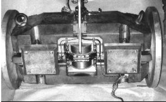
Fig.2: Magnetic system of three-pole BAM-WLS
