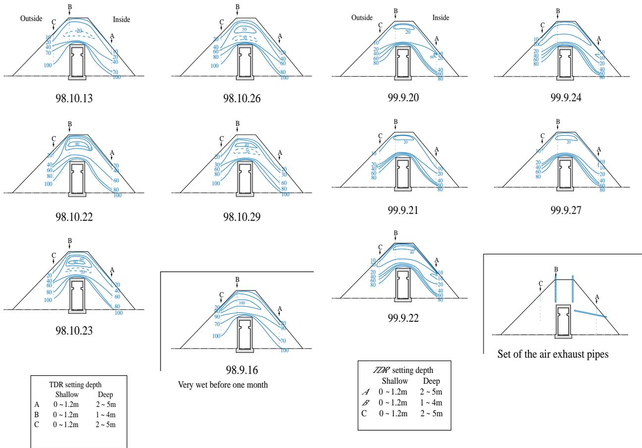
Figure 3: Contours of moisture in the soil bank in October 1998. It was rain of 27.5mm and 12.5mm for September 21 and 22. Just after rain, moisture of soil above the tunnel was only 40% and decreased to that of the bottom by the obstacle of the confined air above tunnel.
