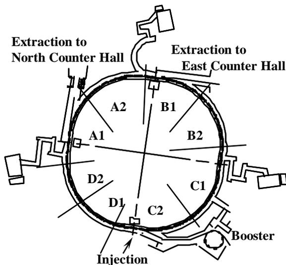
Figure 1. The main ring tunnel comprises eight separated floors.
