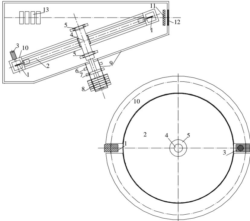
**Figure 1:** Layout of neutron target. 1 - graphite plates; 2 - titanium disk; 3 - bolometer; 4 - shaft; 5 - bearings; 6 - vibration pick-up; 7 - magnetic sensor of rotation; 8 - magnetic clutch; 9 - vacuum chamber walls; 10 - cooling channels; 11 - capacitance-type sensor; 12 - neutron beam output window; 13 - collimator
