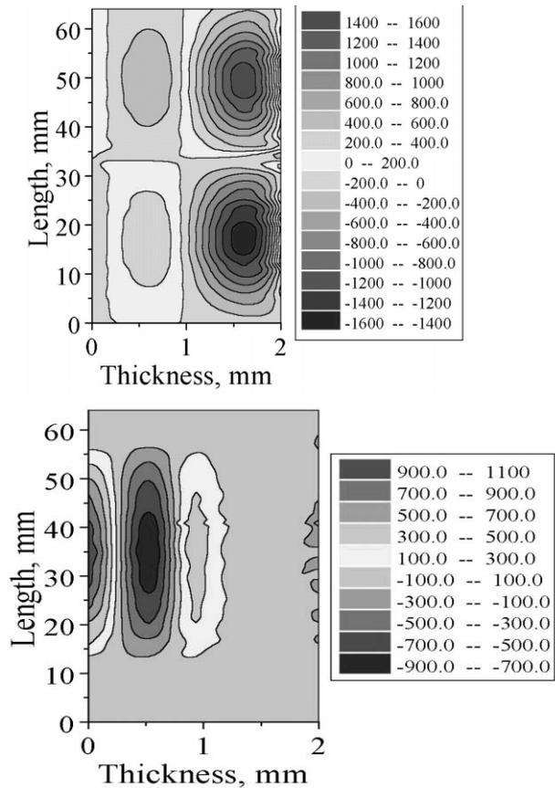
**Figure 3:** Distribution of tangential (above) and longitudinal (below) thermal stress (kPa) over the radial section of graphite for temperature distribution, presented in Fig.2
