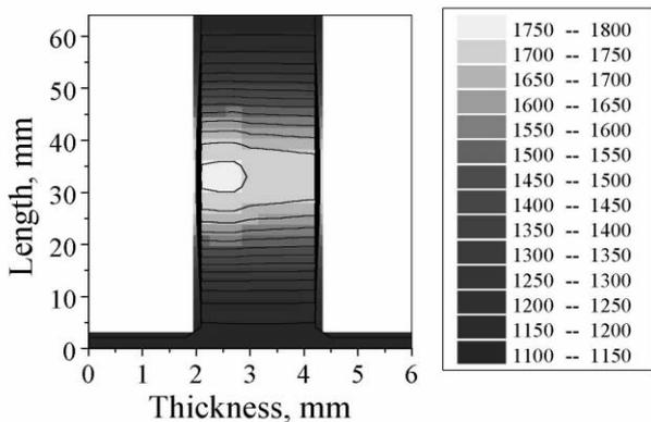
**Figure 2:** Temperature distribution over the section of graphite target in  $^{\circ}\text{C}$  for the graphite length 64 mm and disk thickness 1 cm
