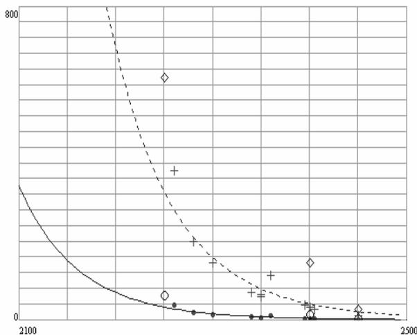
**Figure 4:** Dependence of samples lifetime (hours) on temperature ( $^{\circ}\text{C}$ ). • and O - measured values, + and  $\diamond$  - same values multiplied by factor 10, solid line - approximation, dashed line - approximate values multiplied by factor 10.
