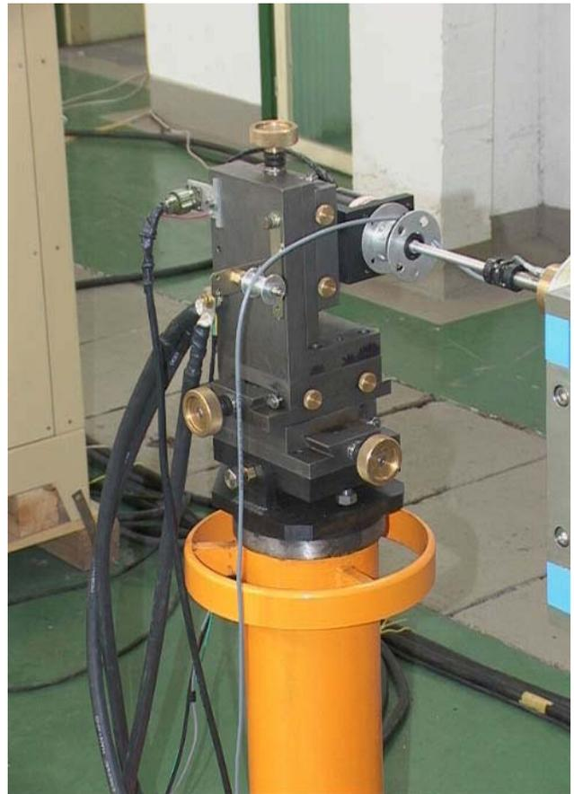
Figure 4: Motor holder of the rotating coil magnetic measurement system
